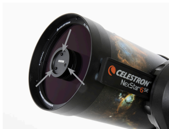
Secondary Mirror Collimation Adjustment Screws
