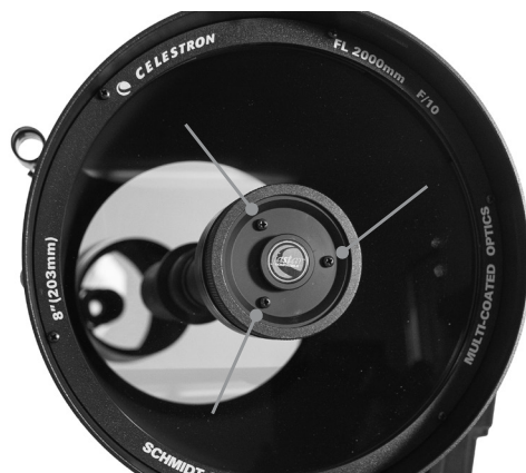
Secondary Mirror Collimation Adjustment Screws
