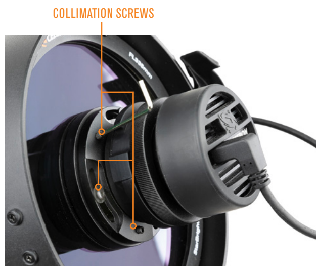
FIG 34: Adjust the tilt of the lens group (and camera) with the collimation screws.
