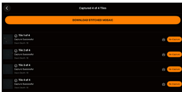
FIG I5: Recapture a tile with the Re-Capture button to the far right of each tile. Download a tile into the app by tapping the download icon to the right of each tile.
