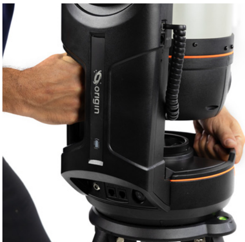
FIG 31: Use the handles on the fork arm and mount to lift Origin.
