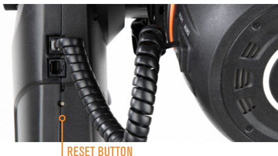
FIG 37: In rare instances, you may need to depress this recessed button to turn Origin off
