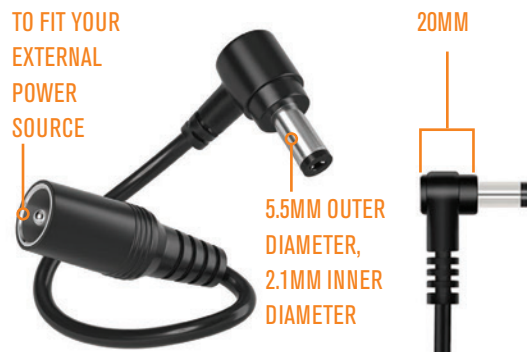
FIG D5: If using external power in EQ Wedge mode, consider purchasing a right-angle adapter for Origin's power jack to prevent the power source's plug from getting pinched between Origin's base and the wedge. This can most often occur at latitudes above 35°. The height of the adapter should be no more than 20mm, and the adapter's plug should have a 5.5mm O.D. / 2.1mm I.D. barrel connector.
