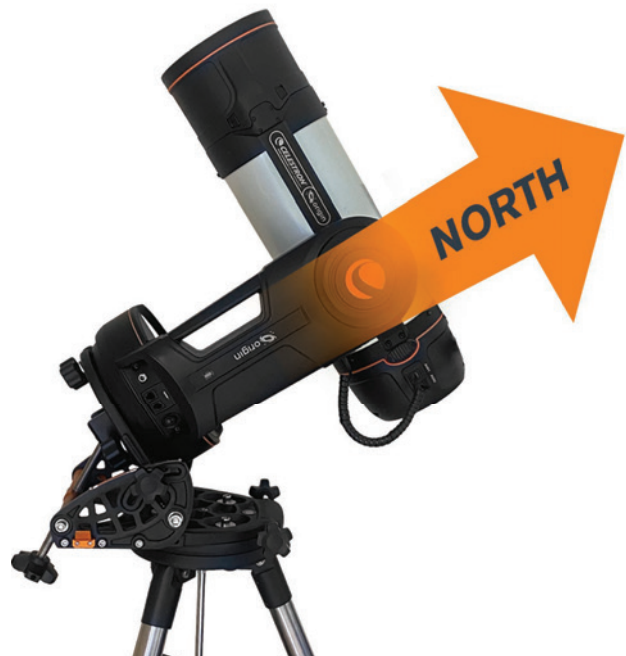
FIG D1: The base of the wedge and the fork arm should be pointing North. If you are in the Southern Hemisphere, the fork arm should be pointing South.
