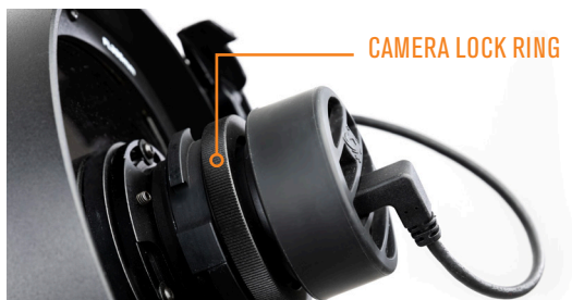
FIG 30: If you wish to rotate the camera orientation, first loosen the camera lock ring.
