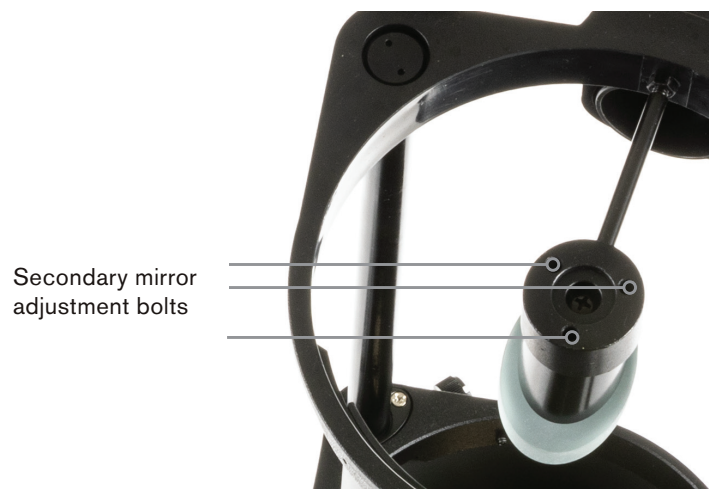
Fig. D: Location of secondary mirror adjustment bolts
